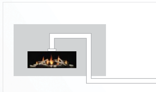
End of line flush horizontal Power Vent system shown in a negative vent run
